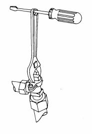
To shut off your water at the meter, first go to your water meter box, which is usually located in front of the house, near the curb. Locate the hole in the plastic cover and carefully lift the cover aside to expose the water meter. Once you have the meter lid opened, locate the customer shut-off valve. Turn the customer shut-off valve clockwise one-quarter turn to the closed position. Attempting to shut off the valve by turning it counterclockwise will destroy the valve.
