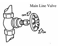
The main supply line to the house usually has a shut-off valve located near where the line enters the building. All valves close with a clockwise turn.
